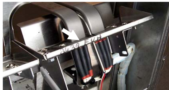
Figure 3: A shroud is provided in the retrofit kit and should be added if the raised edge (shown with the arrow) is absent from the fryer being retrofitted. A tilt-plate without the needed shroud is shown below.
